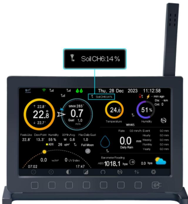
**Figure 35: Data on Main Dashboard of HP2560**
