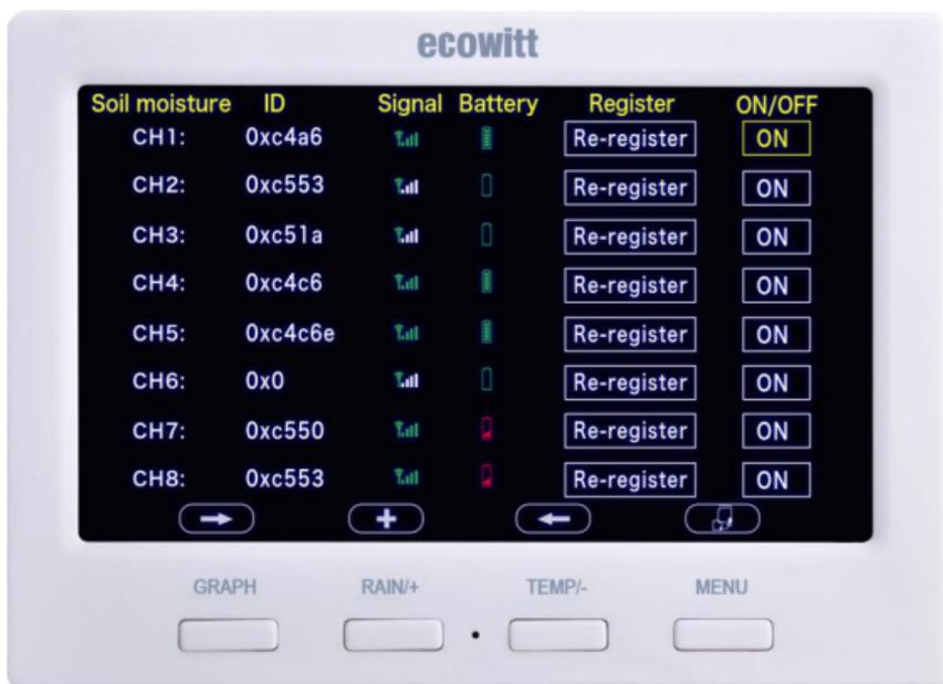
**Figure 39: Register WH51L on HP3500 Display Console**
