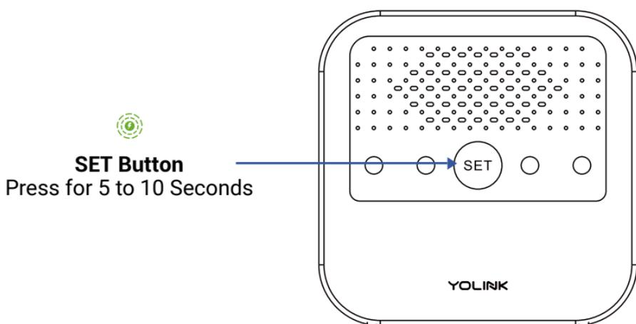
3. Upon pairing, the LED will stop blinking (this may happen after only blinking two or three times).
