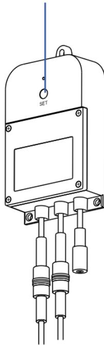
**3.** Upon pairing, the LED will stop blinking (this may happen after only blinking two or three times).
