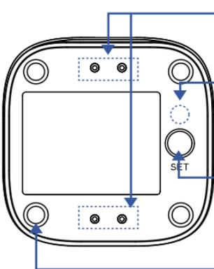
Electrodes (Water Detector)
